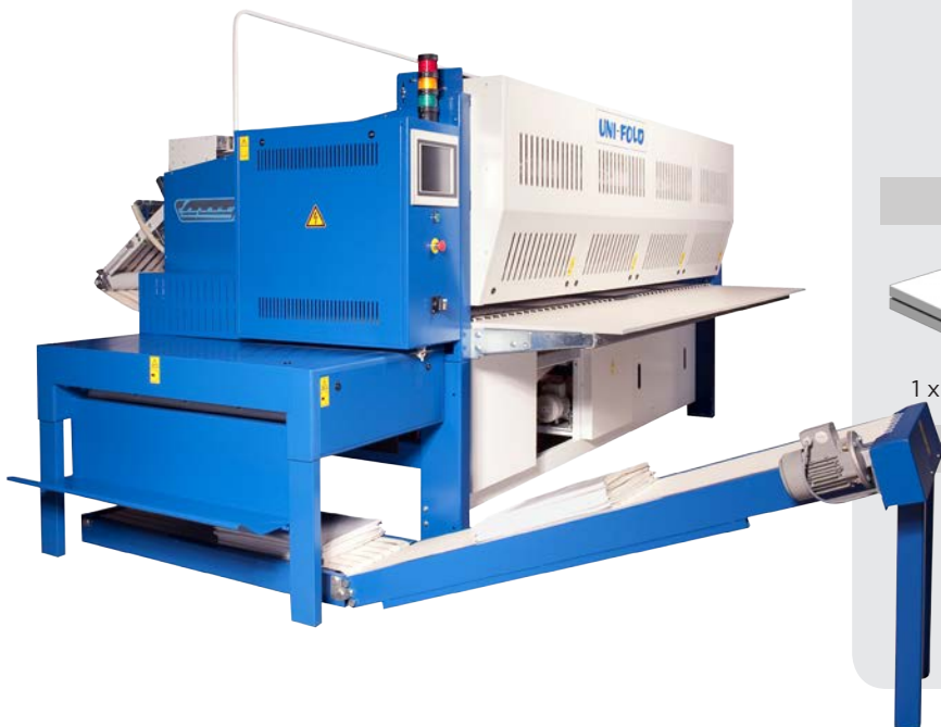
Reliable cross folding: Unifold has knife folding for all crossfolds.
