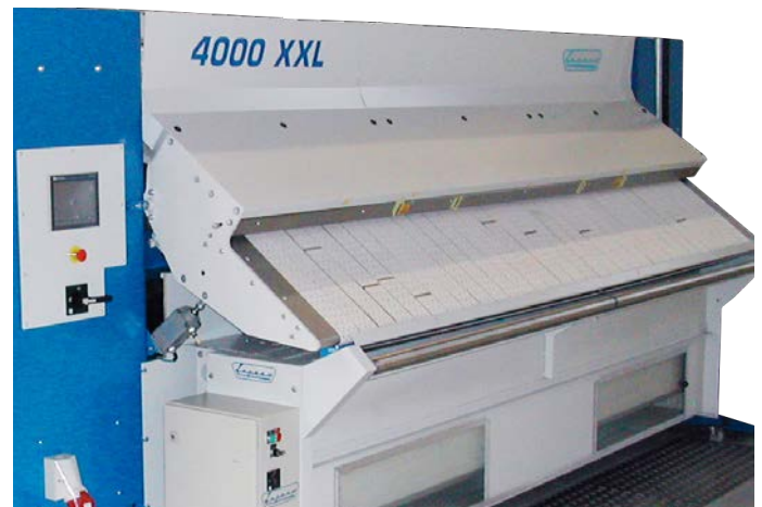
Perforated feedbands with adjustable speed
